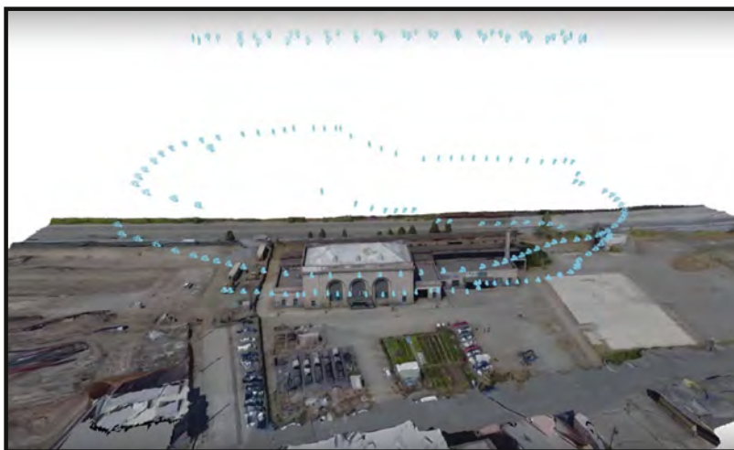
This screen cap shows a flight path around a building exterior captured with 3D scanning and UAS photogrammetry, processed with Autodesk ReCap 360.
